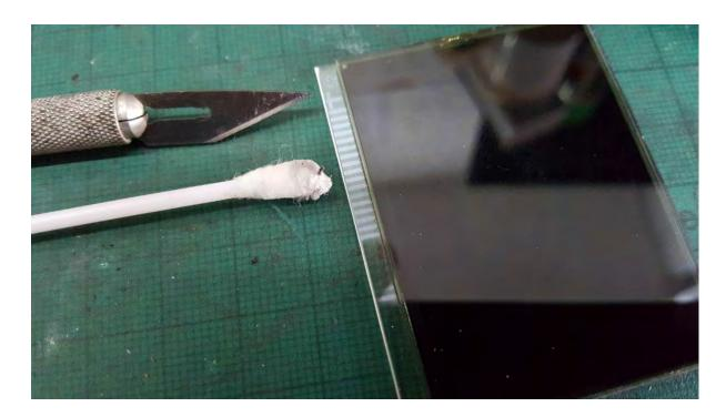
If you hold the LCD display up to the light at the right angle, you can see the embedded electrical contacts in the glass (the lines in the bottom of the glass in the above picture)
