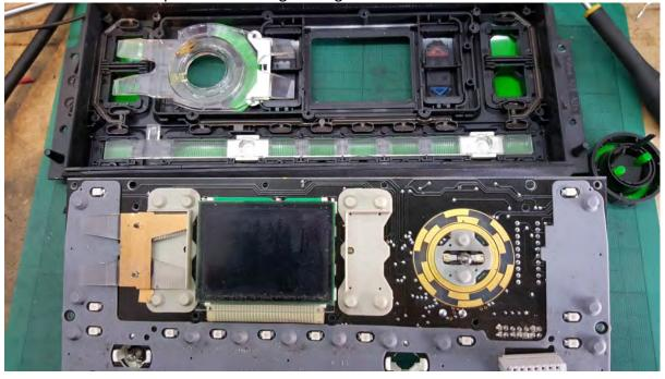
A note here... in the top/left of the picture, you can see the clear plastic light pipe, with the sliding ring in the middle. This is the bit that adjusts the fan speed. The little metal wiper can get tarnished, so if you fan speed knob has been a bit temperamental or you have to
