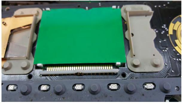
Then fit the new LCD screen connector:
