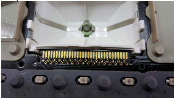
Now is a good time to give the rest of the front panel a clean. The rubber button pads do come off, so you can clean these, and underneath them. They are then fitted back to the board, and there are little rubber 'studs' that push into holes in the PCB to hold it in place.
