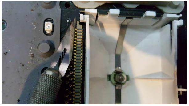
Being careful not to damage the contacts on the board itself. Again give it a clean after removing the remains of the connector:
