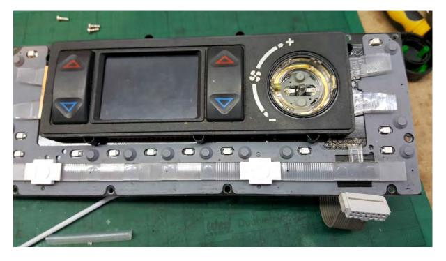
Then carefully overlay the outer part of the front panel. I usually at this point hold the whole thing from the back with one hand, and then fit the front piece with the other, keeping it all flat to avoid everything moving around!
