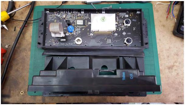
You should then be left with just the front panel. Again, there are now 8 screws holding the PCB into the plastic panel. You can see them removed in the picture below, with the white markings around the outside of the screw head:
