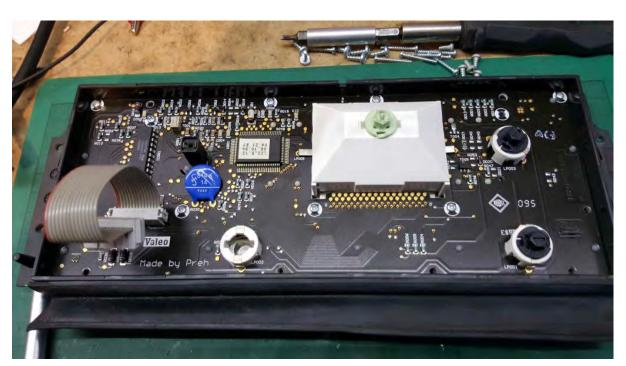
This is also a good time to replace any faulty backlight lamps, before you get the rest of the unit reassembled. Once you are happy everything is aligned, and tight, then you can replace the back plastic cover, and do up the Philips screws around the outside again:
