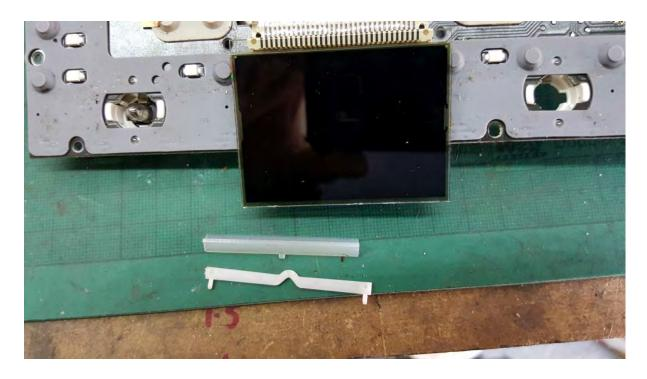
You can now peel the original connector off the PCB:
