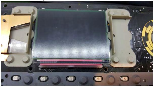
I then re-fit the plastic light pipes and fan knob surround carefully placing them on the PCB, and then refitting the centre section of the front panel over the screen, to make sure everything is aligned properly. It can be a bit fiddly, but most of the plastic light pipes etc all have some form of locating tab(s) so you can't really get them in the wrong place, or assemble it all without them being located correctly:
