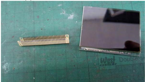
Note the remains left on the LCD glass and the PCB. This will need to be removed with a sharp blade, and some rubbing alcohol to clean the surfaces, before we install the new connector:
