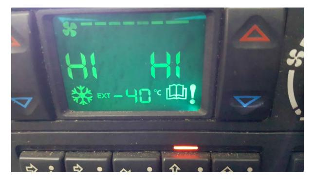
But hopefully without the 'book' symbol and the '-40'. These were showing up in this picture as I was testing this one on the bench, so none of the blend motors/sensors were hooked up! (the other random light bleed in this picture is from the temporary light source I was using, as the backlight lamp had blown in this particular unit, and it became my guinea pig for LED backlighting the display)
