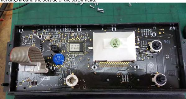
With these removed, you should be able to carefully remove the whole PCB from the casing. I usually put a couple of fingers on the LCD screen to gently get it started moving. If it isn't moving, then double check ALL the required screws are removed!
