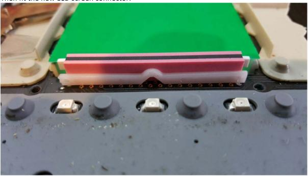
Then the LCD Display on top — making sure you have it up the right way. I give the LCD display a clean before re-fitting with some standard screen/glass gleaner:
