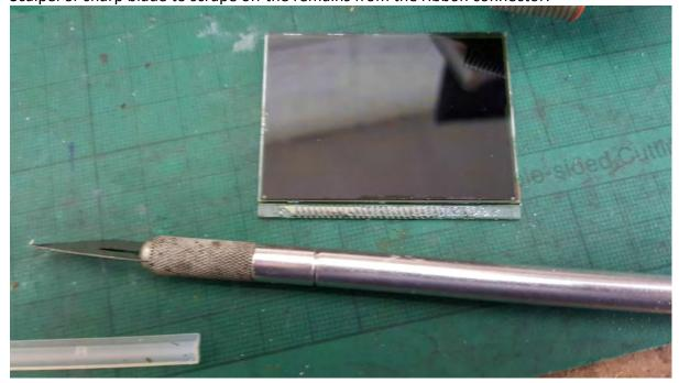
Very carefully scrape the remains from the LCD screen, and then wipe clean with the cotton bud/rubbing alcohol. Be careful not to scratch the conductive etching on the LCD glass, as this can damage pixels aswell!
