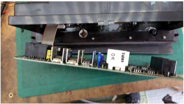
Next, disconnect the ribbon cable from the main PCB that goes to the front panel:
