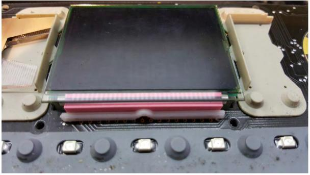
Make sure the connector is centered along the display, so that all of the electrical connectors are covered by the black core of the connector:
