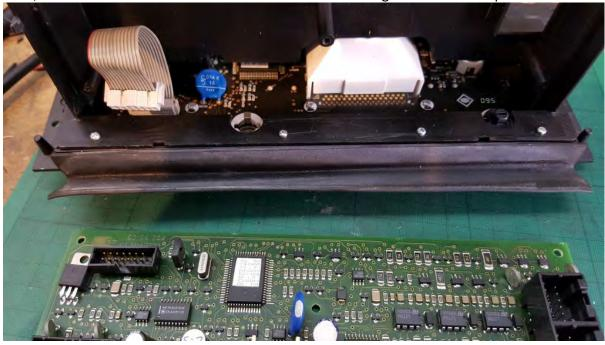
Set the main PCB aside with the bottom metal cover, and the screws in a safe place, ready for re-assembly.
