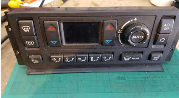
First, start by turning the unit upside down, and removing the 6x Torx head screws from the bottom panel:
